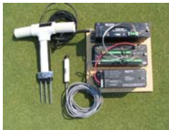
Figure 2. TDR device and datalogger used for measurement and storage of volumetric water content data of the field sites.
